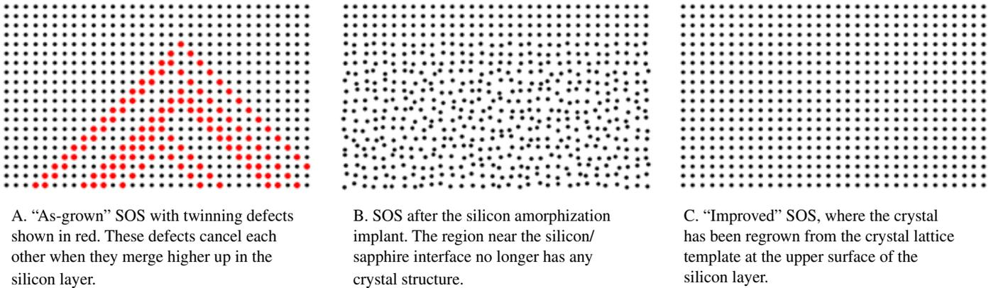
**Figure 3.** A schematic representation of the Solid Phase Epitaxial Regrowth (SPER) process.
