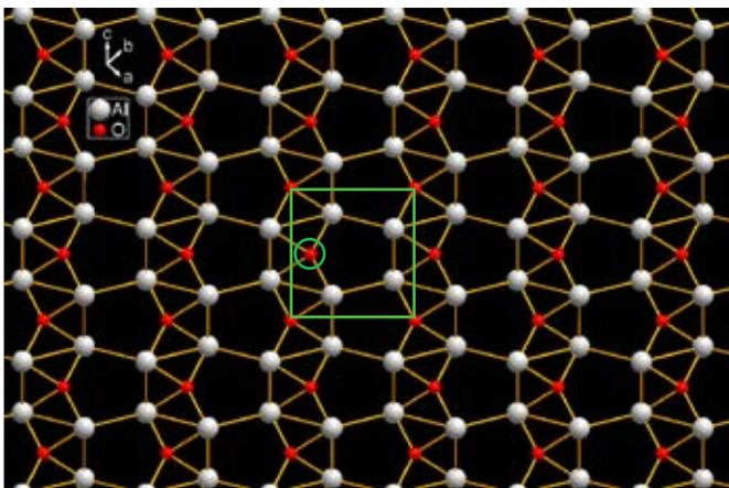
**Figure 1.** A view of the r-plane of sapphire. The green box illustrates the square symmetry of the oxygen atoms. The green circle shows the extra oxygen atom that is used in the SiO<sub>2</sub> bond. The yellow rods represent atomic bonds.
